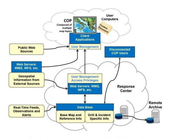
Figure 10: OSR Common Operating Picture (COP) delivery architecture
