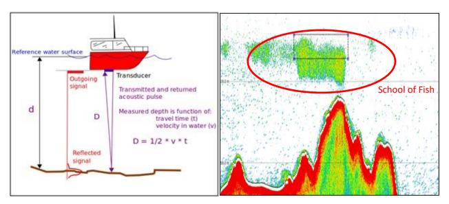
Figure 7. Example of estimating depth with a simple echo-sounder (left), and illustration (right) of the potential for blunders (e.g., the echo-sounder detecting the depth of a school of fish, rather than the seafloor).
