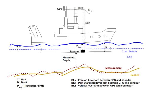
Figure 12. Effects of not correcting for horizontal offsets. Here, not measuring the horizontal offset between the GNSS receiver position and the echo-sounder results in along-track offsets of seafloor features. Red line: measured; yellow line: reality.
