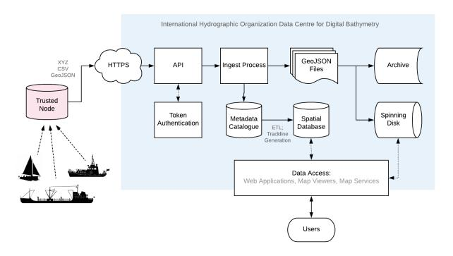
Figure 3. A schematic of the flow of CSB data from the Trusted Node, to the IHO DCDB, and to the public.
