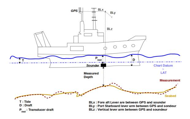
Figure 10. Effects of accurate, but not precise uncertainty on a depth sounding. Here, on average the depth measured (red line) is correct but point to point it varies from the true depth (yellow line).
