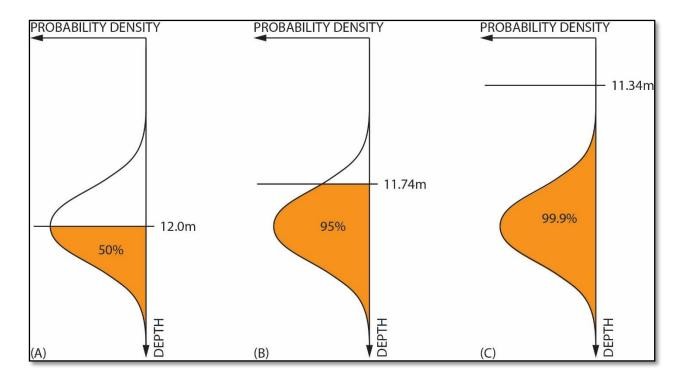
Figure 13. Examples of shoal-clearance depths for different probabilities of excession, based on the same basic uncertainty estimate of  $12.0 \pm 0.3$ m (95% CI). Assuming a 12.0m clearance is only true 50% of the time (left); a 5% probability of being shallower requires the depth to be reduced to 11.74m (middle); a 1:1000 chance of being shallower requires a clearance depth of 11.34m (right).
