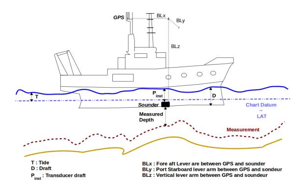
Figure 11. Examples of the effects of not correcting for vertical offsets. Here, not correcting for the offset of the transducer from the waterline leads to a measurement (red line) that differs significantly from reality (yellow line). This gives a bias (systematic) uncertainty to the measurements.
