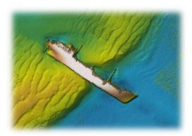
A wreck detected by side scan sonar
