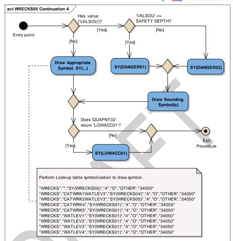
Figure 434344 WRECKS05 Continuation A
