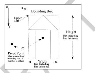
Fig 2. Pivot point, bounding box and symbol coordinates.
