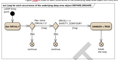
Figure <u>393940</u> Loop for each occurrence of the underlying deep area object DEPARE,DRGARE
