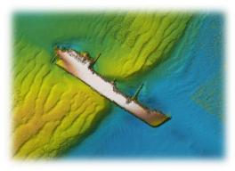
A wreck detected by side scan sonar
