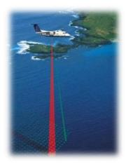
**Airborne laser depth sounder**. Light Detection and Ranging (LiDAR) systems using a laser in an aircraft to measure depth can provide substantial productivity gains for surveys in shallow, clear water. LiDAR systems are capable of measuring depths up to 50m or more in optimal conditions where the water is relatively clear. LiDAR survey services are usually provided to governments by private contractors.
