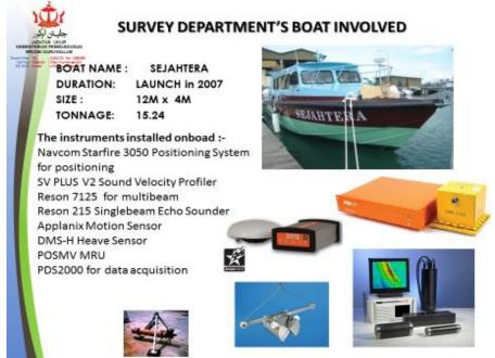
Survey platform and equipment used in hydrographic survey (Source: Hydrographic Unit presentation)
