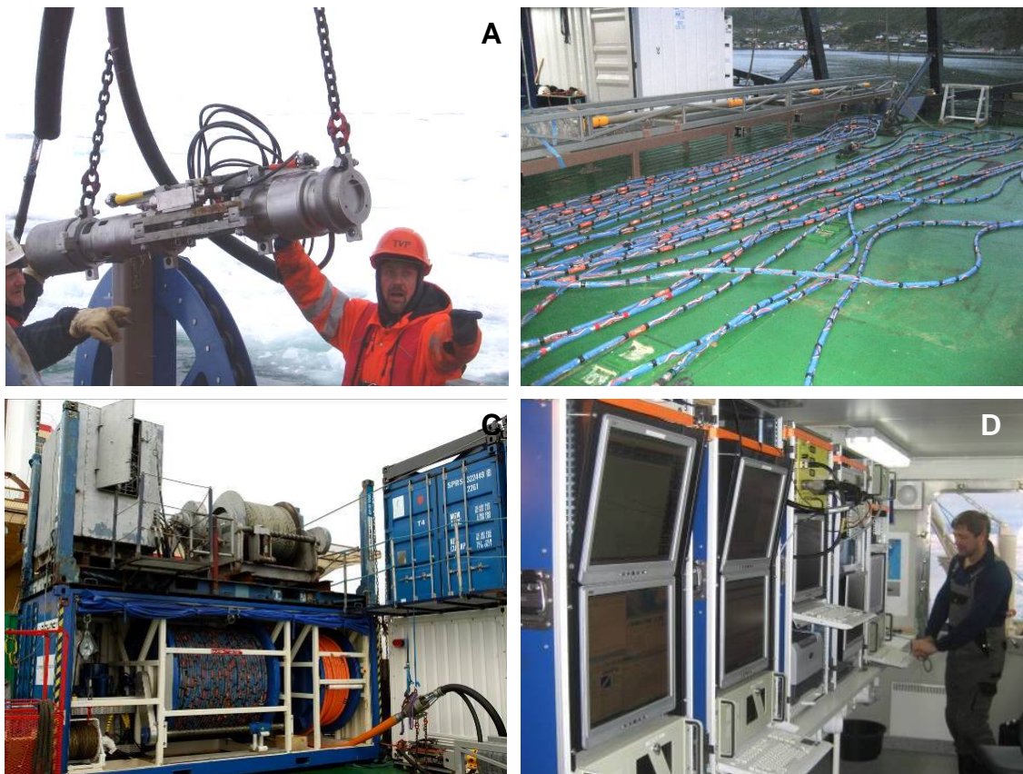
Figure 12: Seismic equipment developed for acquisition of seismic data in heavy ice conditions within the Danish Continental Shelf Project. In order to minimize the risk for ice induced physical damage of the equipment towed in the water behind the icebreaker and to reduce the risk for having the streamer forced up towards the ice by propeller wash the tow depth was increased to calm waters below the propeller wash at a depth of approximately 20 m. The choice
