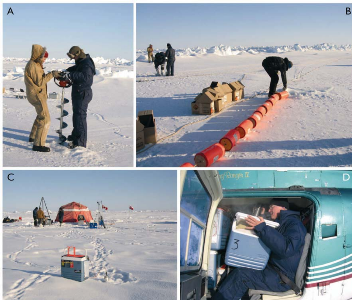
Figure 7: LORITA refraction seismic experiment spring 2006. A – Each seismic line required drilling 11 holes approximately 20 Km apart. B – Suspending either 350 Kg or 175 Kg of Pentolite explosives 100 metres below the ice at each hole. C – Setting out up to 100 seismometers at intervals of 1.5–2 Km and firing the charges. D – Collecting all the instruments and then downloading the data (Photos: Christian Marcussen and Ron Verrall).
