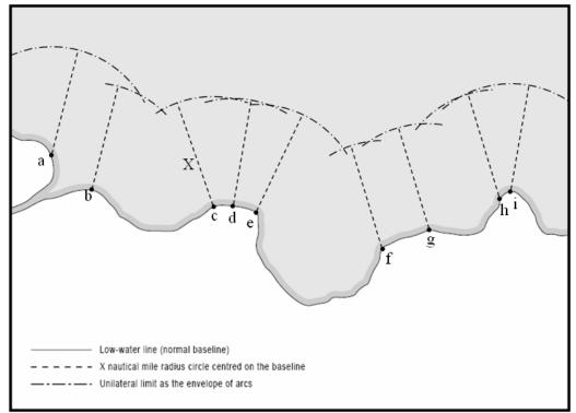
Figure 2 Envelope of arc and relevant basepoints
