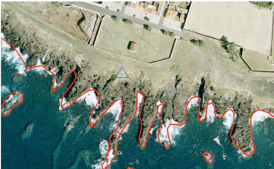
Figure 5 – Assessing the positioning quality of the data after applying the new referencing systems.
