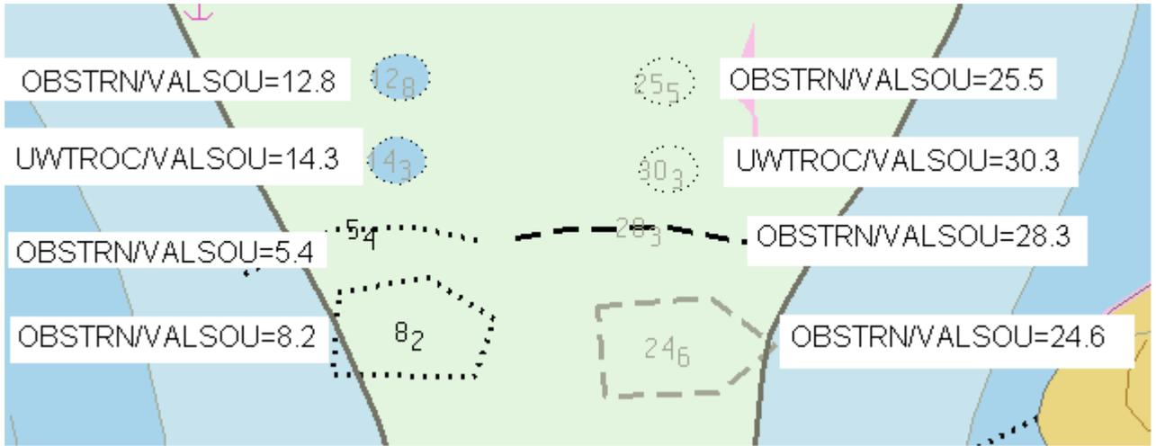
Diagram 1: Testing drawing of soundings on top of OBSTRN/UWTROC features (points, lines and areas).
