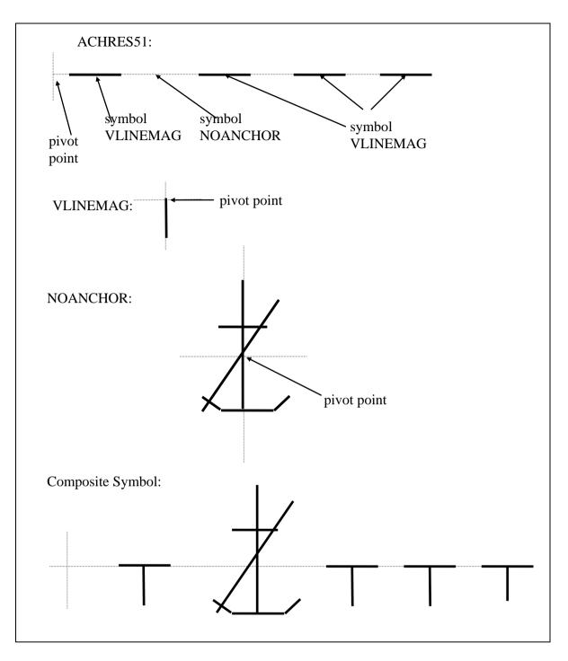
3. Re-number "Fig. 3-Usage of complex linestyle" as "Fig. 3a.-Usage of single unit type of complex linestyle", and add new "Fig 3b-Usage of composite type of complex linestyle" shown abov
