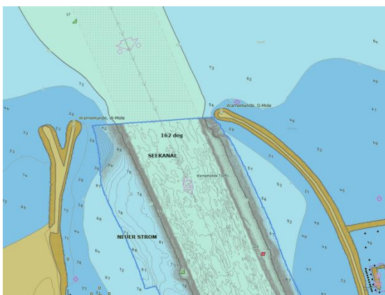
The picture above shows the bENC as a merge of ENC and ABL
