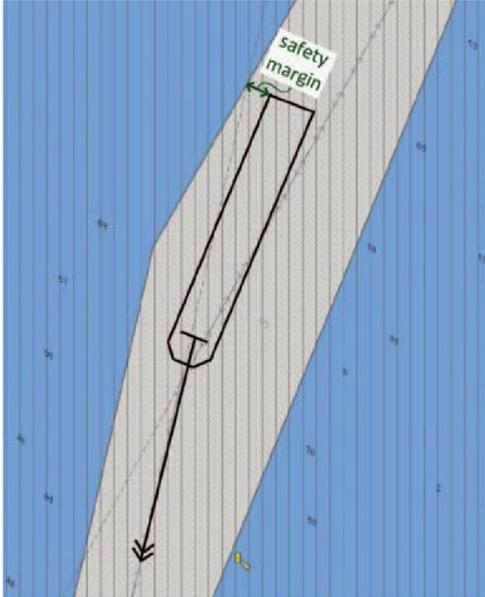
the Harbour ENC provides only an 8.3m maintained depth value that is associated to the dredged area that covers most of the outer harbour
