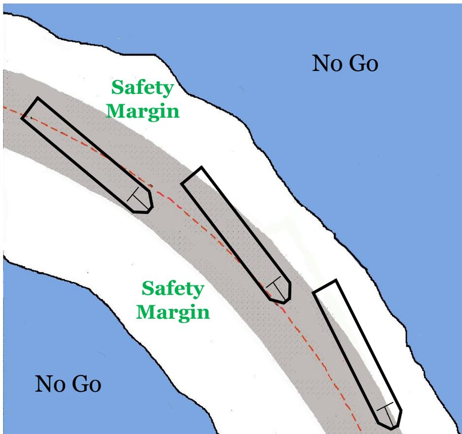
High Density ENC's enable **higher resolution** and **more accuracy** in the visualization of no go areas and, as a result, of the **safety margin**
