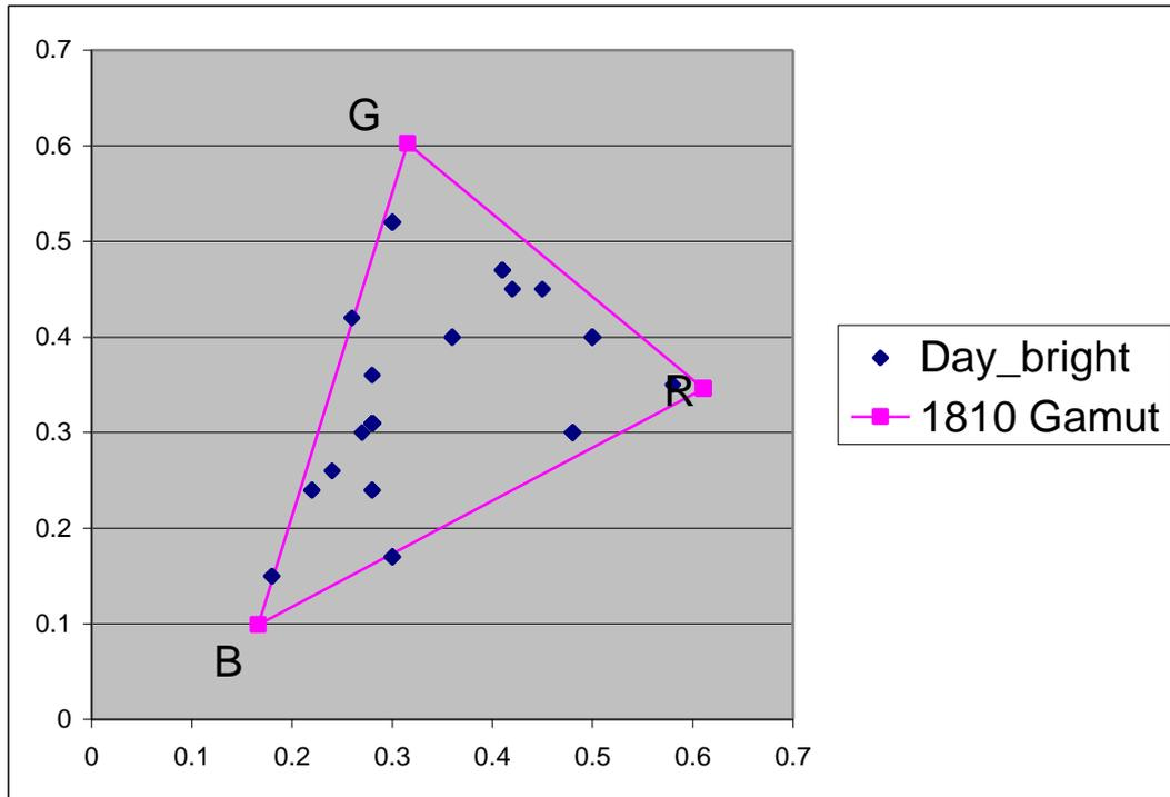
Plot showing the Day\_bright colour table, and that all colours are achievable by the display. Note that there several colours that are marginal in performance – especially along the blue-green line. (These colours are within calibration tolerance.)
