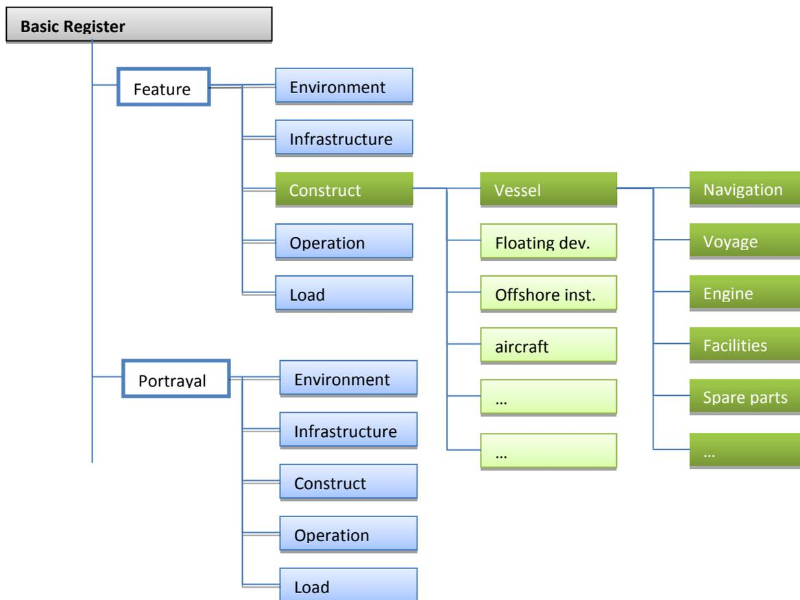
Figure 1: Example for part of the structure of the proposed future “Maritime Information Registry on the basis of S-100
