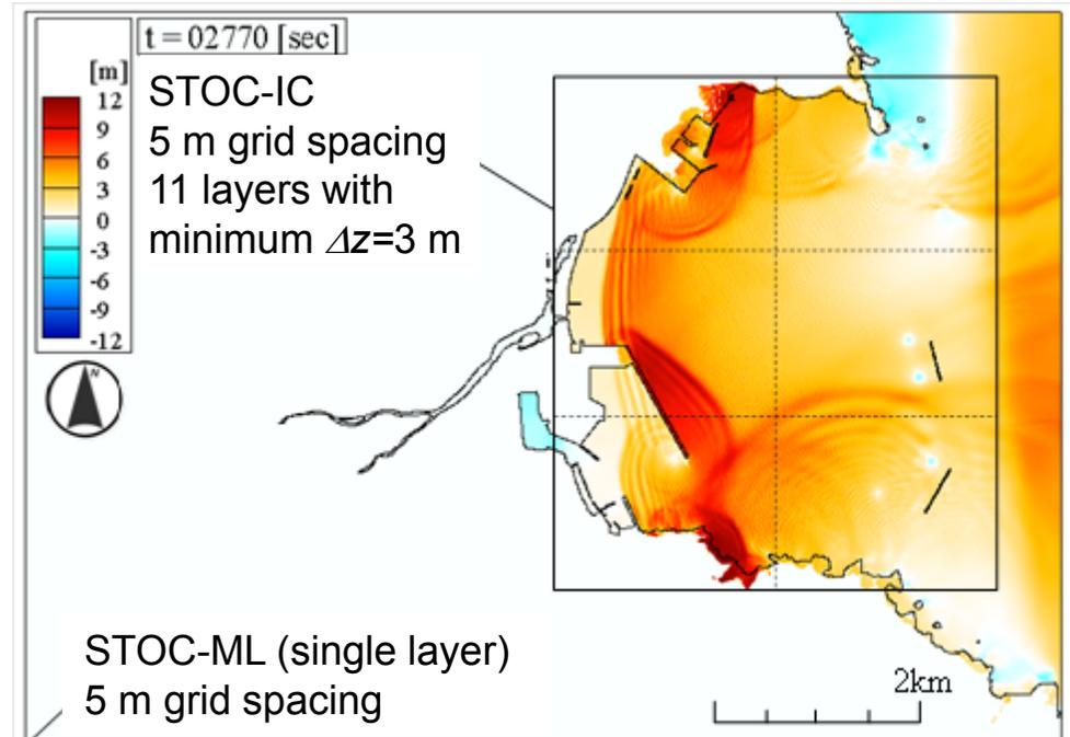
Red strips: Short-period waves on the tsunami front in orange color
