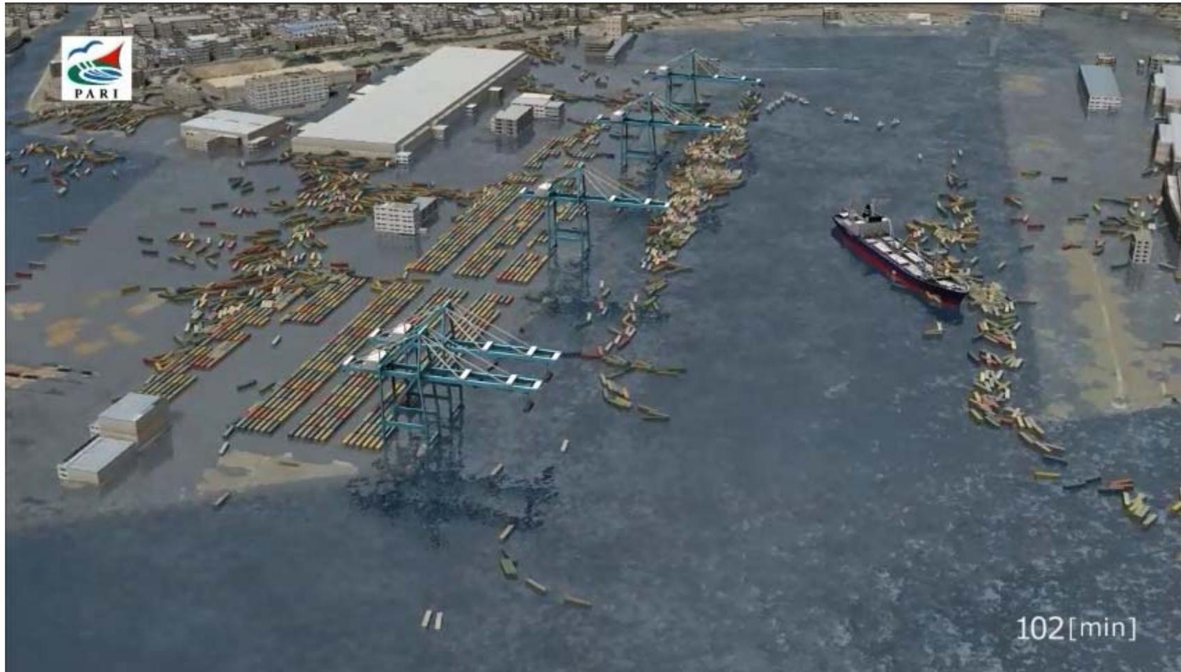
CG of a result of tsunami inundation and debris calculated by a tsunami numerical simulation model of STOC
