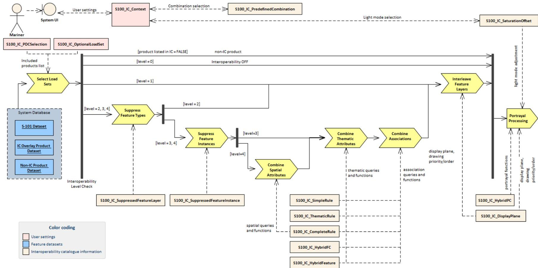
Figure 9. Interoperability processing model – Phase 2 (Option 1 – Interoperability before Portrayal).
