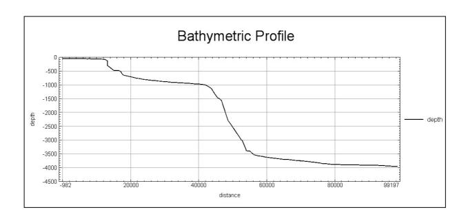
These Cruises were carried out by LEPLAC – The continental shelf survey during 1994 and were acquired by NHi Sirius. The navigation systems used were Racal/GPS/TRIMBLE. The Bathymetric data were acquired employing Krupp Atlas Deso-25.
