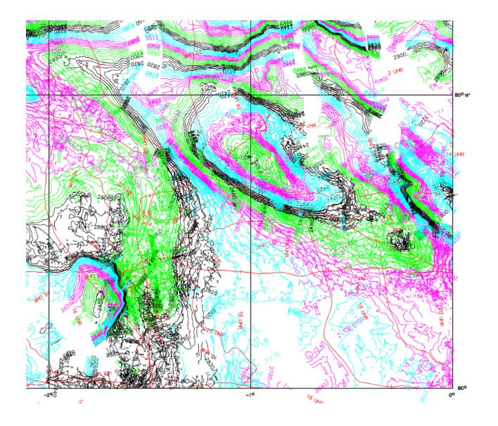
Multibeam Survey of the Koldewey Seamount plus track lines from RV Polarstern
