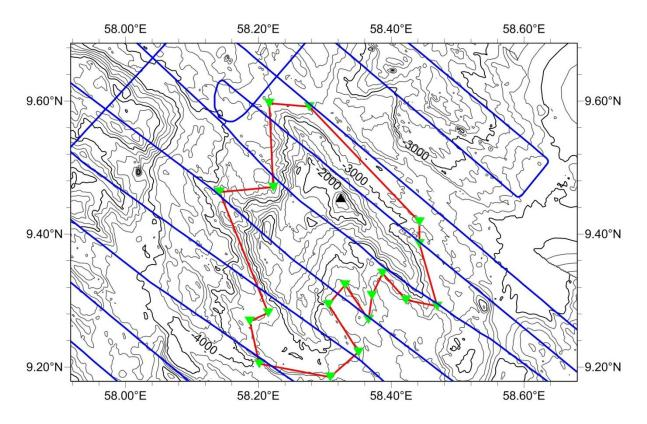
Fig 3. Isobath and survey line map of Wanwu Seamount (Contours are in 200 m, blue lines are survey lines)
