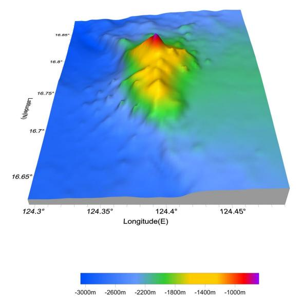
Fig.6 3-D bathymetric map of Qiangde Seamount
