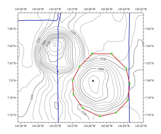
Fig 3. Isobath and survey line map of Luobinwang Knoll (Contours are in 50 m, blue lines are survey lines)
