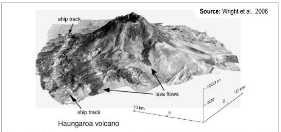
Fig. 11. EM300 back-scatter imagery draped over bathymetry terrain grids (cell size 25 m) for Haungaroa volcanoes. Areas of high acoustic reflectivity (back-scatter) are shown as black/dark grey and are interpreted as recent lava flows, whereas areas of light grey are interpreted as sediment.
