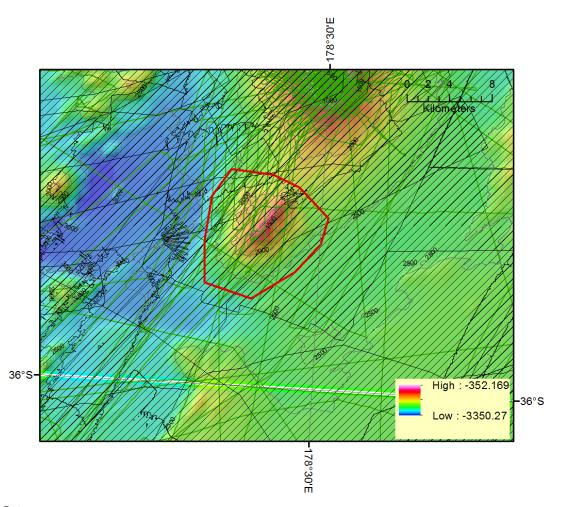
Data coverage Cross-hatch = multibeam bathymetry coverage Dark green = single beam bathymetry data
