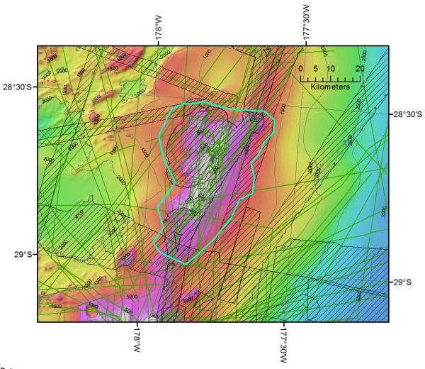
Data coverage Cross-hatch = multibeam bathymetry coverage Dark green = single beam bathymetry data
