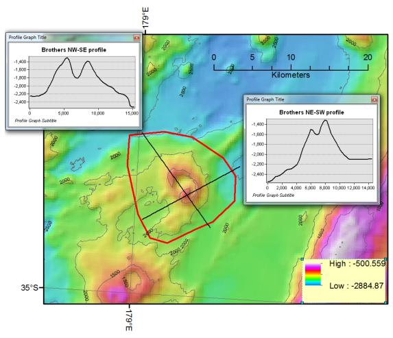
Bathymetry of Brothers Seamount and profiles of the feature. Summit elevation is 1197 m
