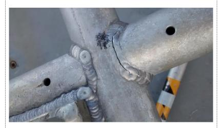
**Above**: One of the fractures sustained during a bad weather recovery. These were also fixed by *Falkor's* engineering team
