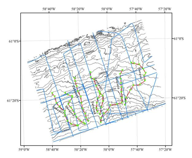
Fig.3 Bathymetric map of Wangjing Canyons overlain with track lines (Contours are in 200m, blue lines for the track lines)
