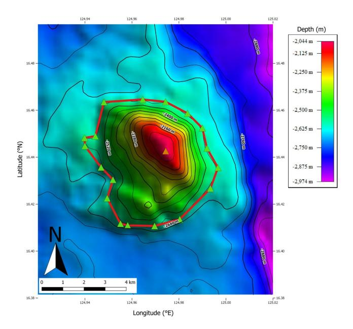
Figure 2. Bathymetric map of the Palosapis Hill. Contour interval is 60 meters.
