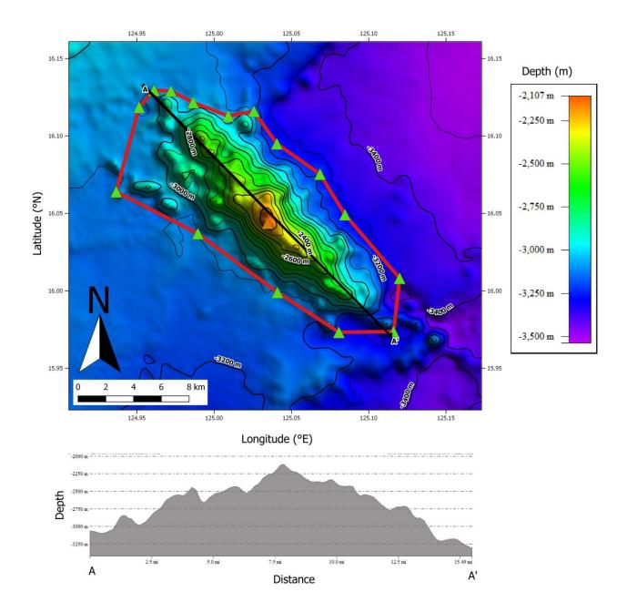
Figure 6. Profile of the Pili Ridge from NW to SE (A to A').
