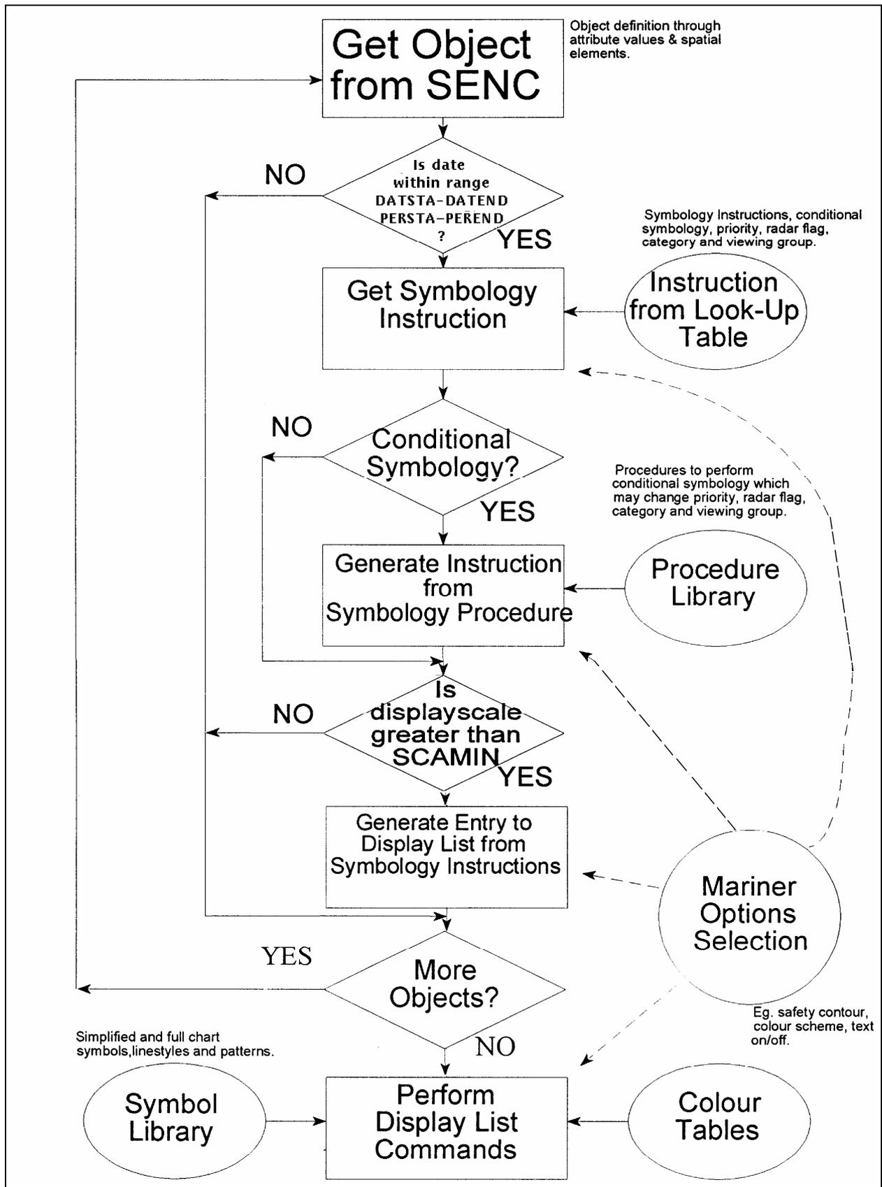
Fig. 1 -Display generator- ECDIS display concept
