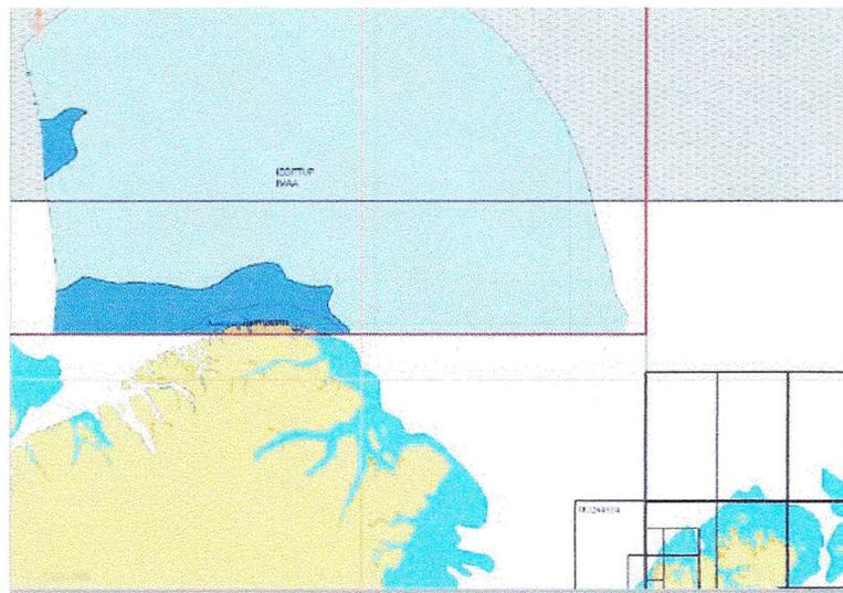
Displaying ENC in area north of 84° N will require a different type of projection, for example a polar stereographic projection. The challenge is that these are not defined by the current IMO ECDIS performance standards.
