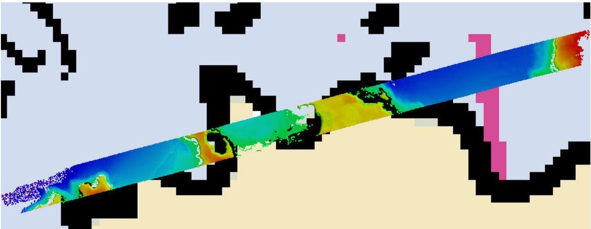
**Figure 6 – Sub-section of CARIS BASE Surface image demonstrating lidar coverage to the NE of Nash Harbor, central north coast of Nunivak Island.**
