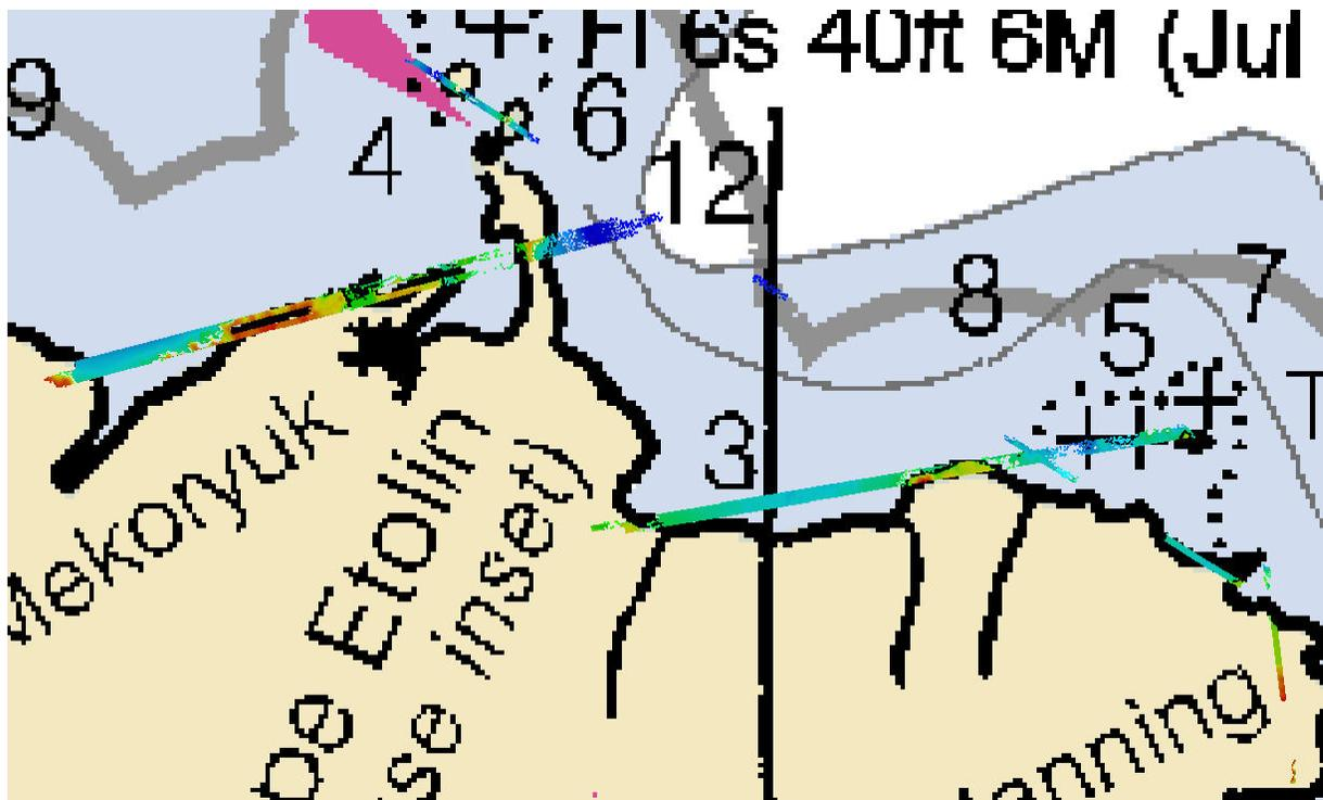
Figure 7 – Sub-section of CARIS BASE Surface image demonstrating lidar coverage from Cape Etolin to Cape Manning, northeast coast of Nunivak Island.
