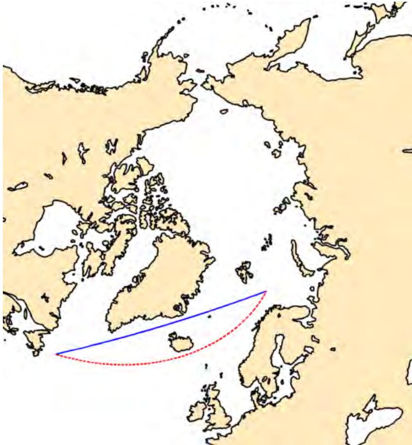
Figure 76. Azimuthal Polar Equidistant projection, Departure point at  $50^{\circ}$  N,  $50^{\circ}$  W, Destination point at  $74^{\circ}$  N,  $28^{\circ}$  E. Orthodromic distance 1550.1 n. m., Loxodromic distance 1557.5 n.m.
