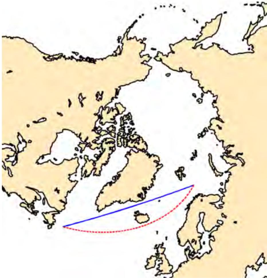
Figure 74. Azimuthal Polar Stereographic projection, Departure point at 50° N, 50° W, Destination point at 74° N, 28° E, Orthodromic distance 1550.1 n.m, Loxodromic distance 1557.5 n.m.
