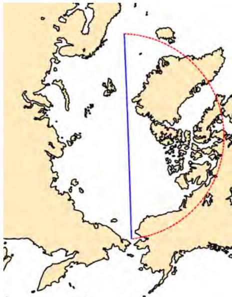
Figure 77 Azimuthal polar Equidistant projection, Departure point at  $67^{\circ}$  N  $169^{\circ}$  W, Destination point at  $67^{\circ}$  N  $3^{\circ}$  E, Central meridian at long  $175^{\circ}$ , Orthodromic distance 2765.6 n.m., Loxodromic distance 4051.1 n.m
