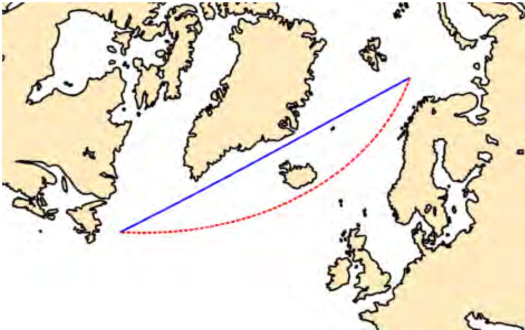
Figure 71. Lambert Conformal projection (standard parallels at latitudes 58 ° and 82°), Departure point at 50° N, 50° W, destination point at 74° N, 28° E, Orthodromic distance 1550.1 n.m., Loxodromic distance 1557.5 n.m.
