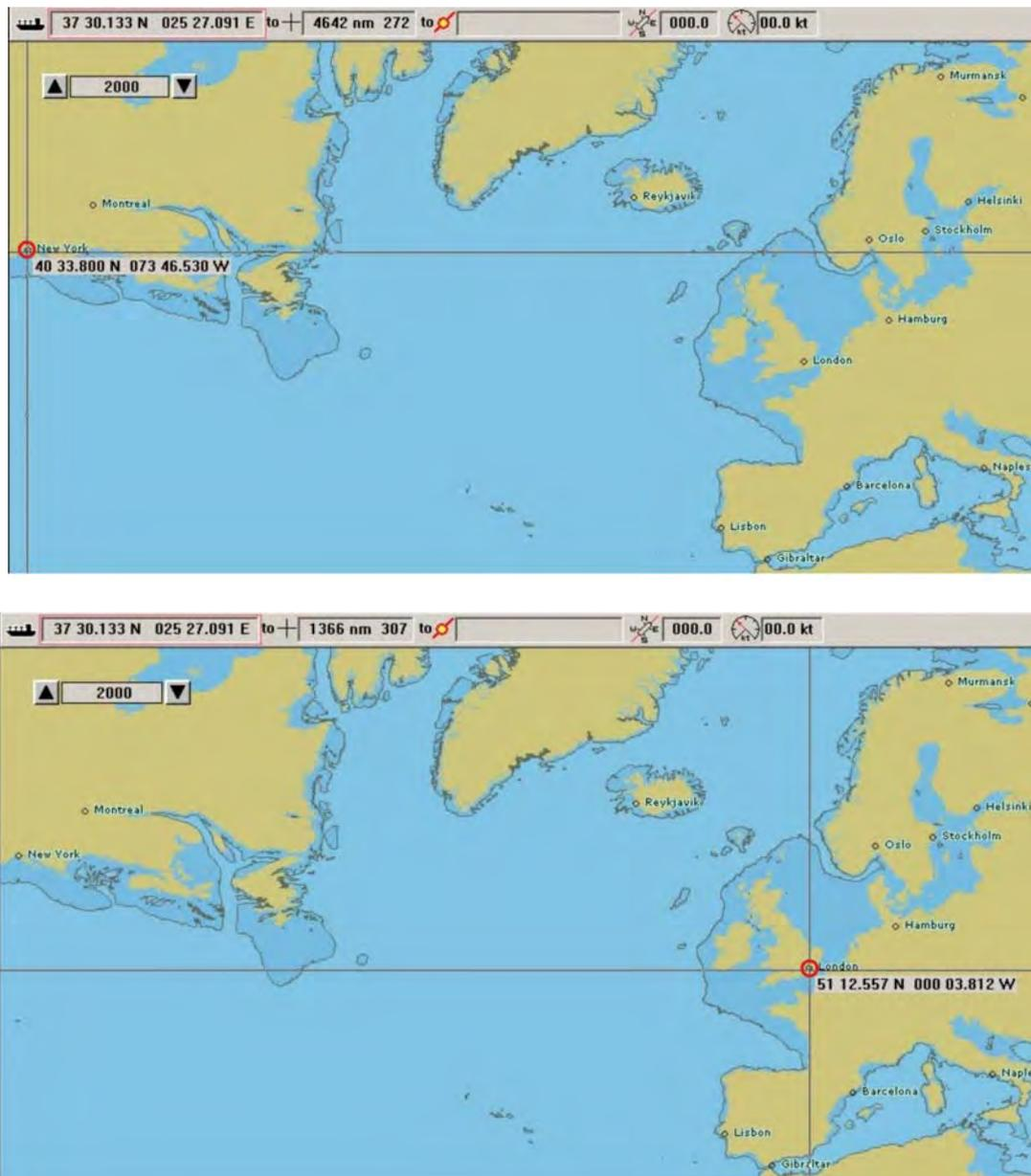
Figure 3. Portrayal of the false impression given in ECDIS when graticule lines are not shown
