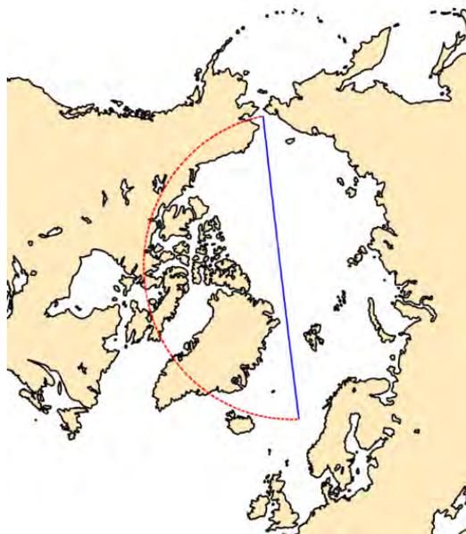
Figure 78. Azimuthal polar Equidistant projection, Departure point at  $67^{\circ}$  N  $169^{\circ}$  W, Destination point at  $67^{\circ}$  N  $3^{\circ}$  E, Central meridian at long  $000^{\circ}$ , Orthodromic distance 2765.6 n.m., Loxodromic distance 4051.1 n.m.
