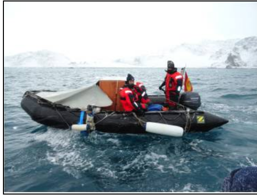
Figure 4. Very shallow water bathymetry system operated from a boat
