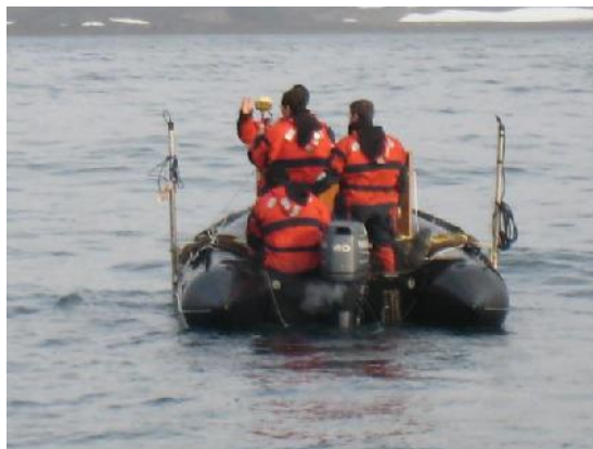
Figure 5. Very shallow water bathymetry system operated from a boat
