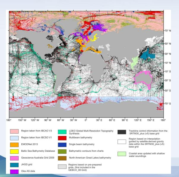
Example of the **GEBCO** Source Identifier (SID) Grid showing the source of depth value in each grid cell, i.e. if it is based on trackline data; pre-existing grids or if it is based on interpolation
