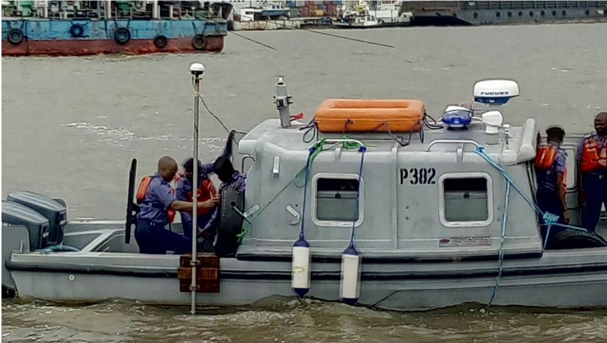
Fig 4. Single beam survey using an EPENAL E-27 Patrol Boat
