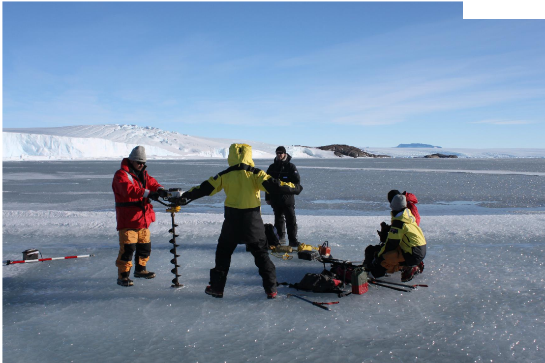
1. Drilling ice holes to take single beam echo sounder reading in the vicinity of Mawson Station, Antarctica
