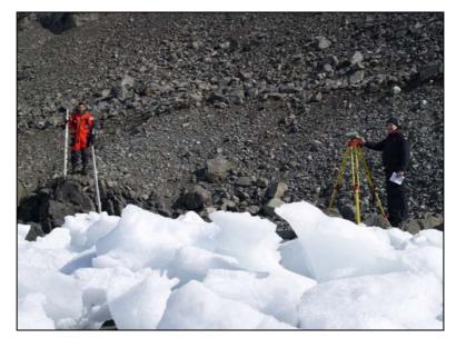
Figure 11. Levelling tide bench marks
