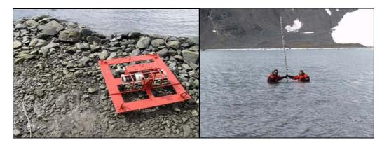
Figure 10. Bottom pressure sensor for tide measuring
