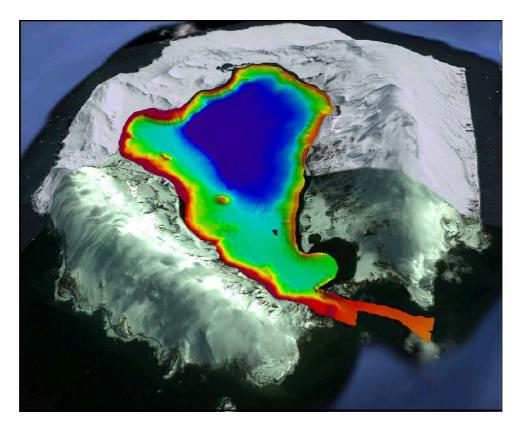
Figure 8. Multibeam survey of Port Foster, Decepcion Island
