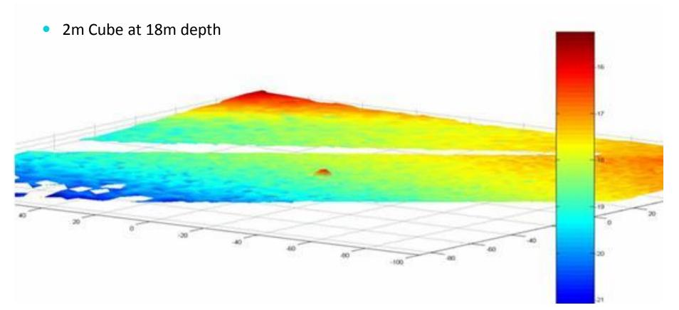
• HEIIb meets the object detection requirement of >2m in up to 40m depths
