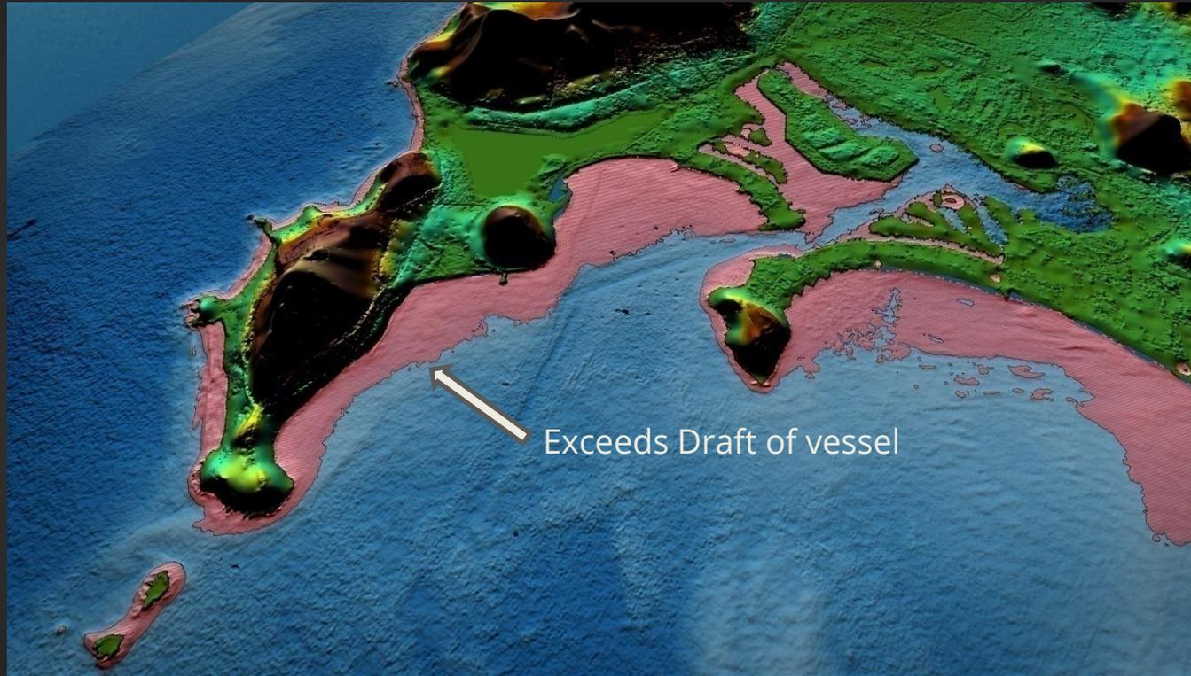
Facilitate landing diagram creation, using hydrographic observations to identify hazards, optimal boat lanes and landing beaches based on craft capabilities and seafloor classification.
