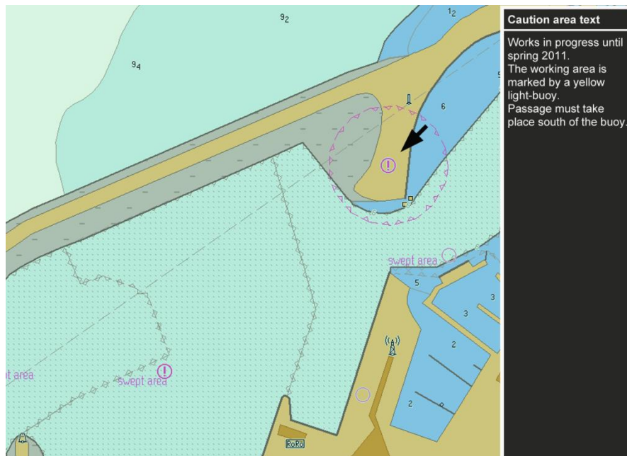
Works in progress in the port of Visby. The affected area is shown in ENC as a “caution area” with associated text.
