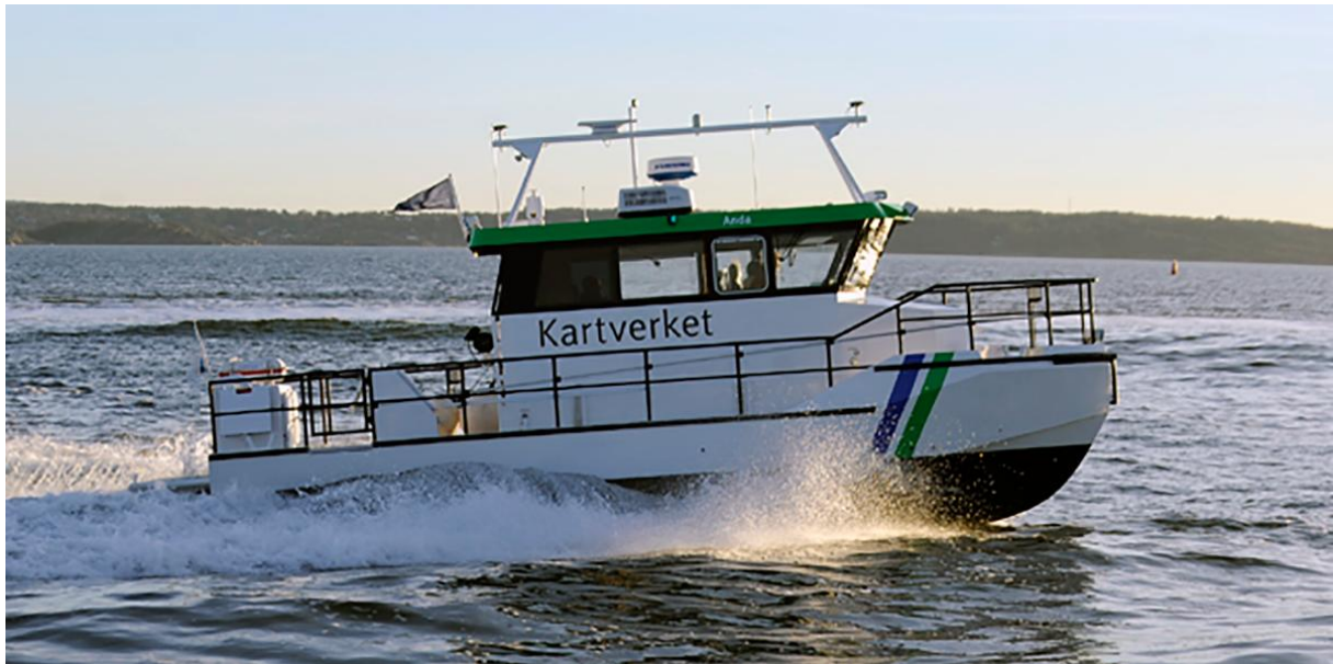
Fig. A new survey launch: Length 11.15m, breadth 3.4m, service speed 25knots, 2 waterjets, EM2040 Dual head MBES, Seapath 330+ motion sensor
