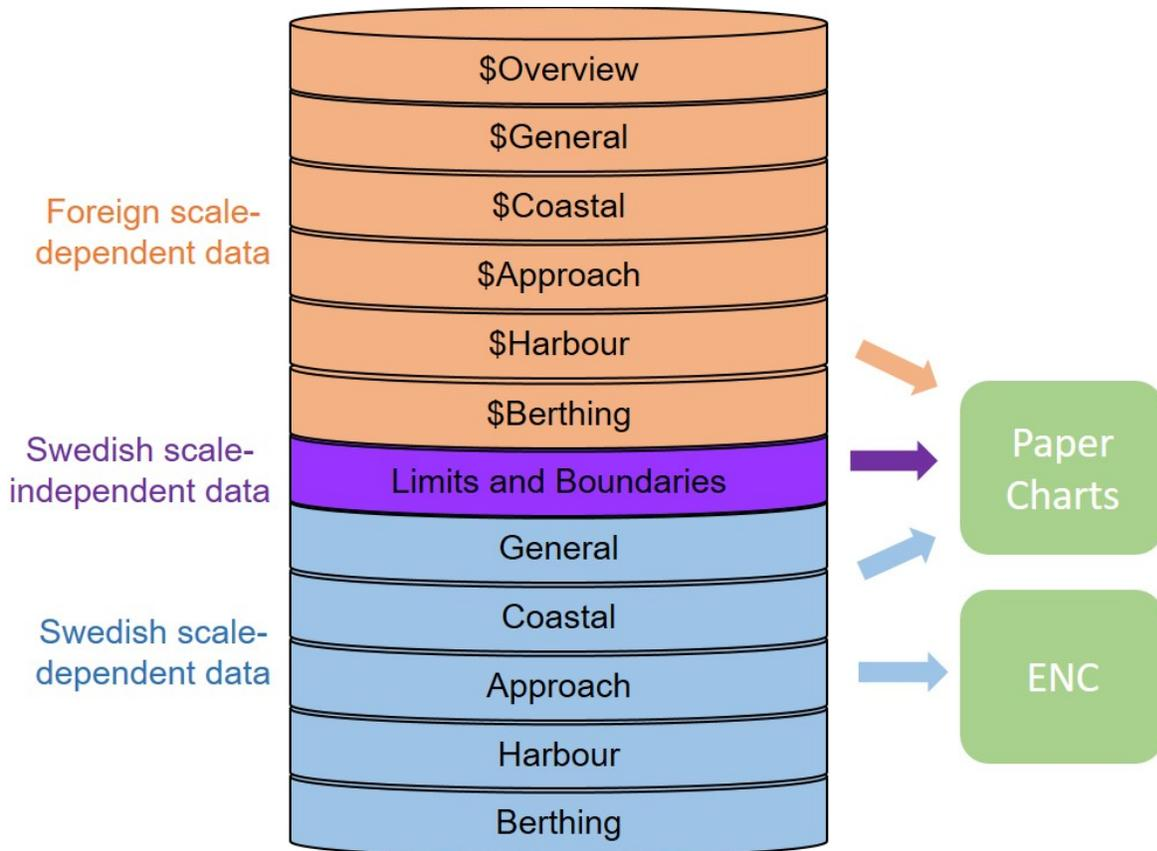
Fig. 4. Structure of SMA chart-production database
